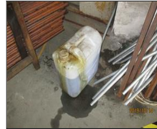
Photo of non-conformity 7.7 No 2nd container and MSDS.JPG
